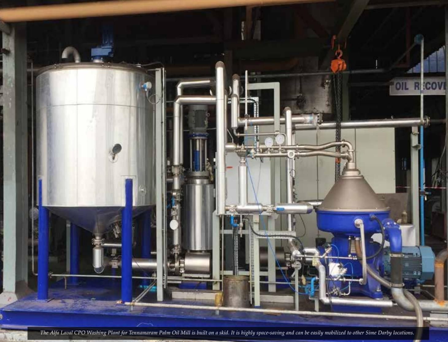
The Alfa Laval CPO Washing Plant for Tennamaram Palm Oil Mill is built on a skid. It is highly space-saving and can be easily mobilized to other Sime Darby locations.
