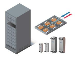
The cold plate is attached to the CPUs/GPUs, the fluid (1 or 2phase) removes the heat.
