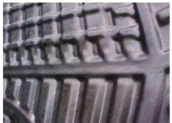
Deformation of the diagonal gasket groove.
