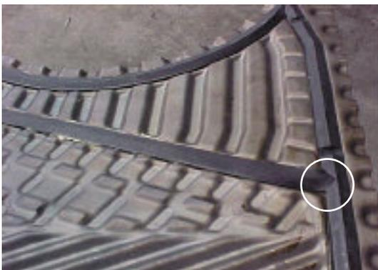
The diagonal gasket has moved from its groove at the junction where it meets the side gasket groove, shown here within the ring.
