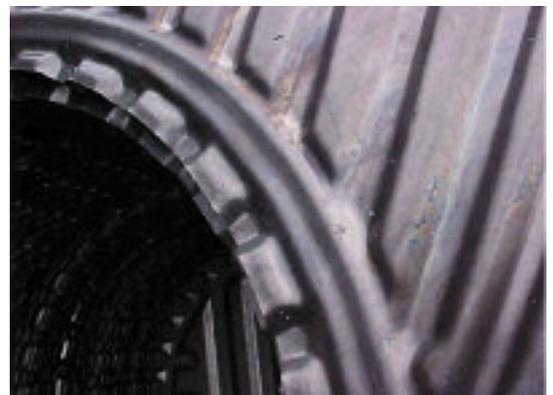
Extensive deformation of a port gasket groove.
