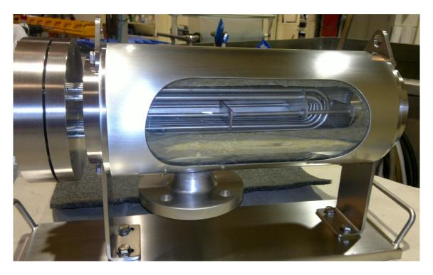
In Alfa Laval Pharma-line we are going beyond the ASME BPE recommendation for bending radius
