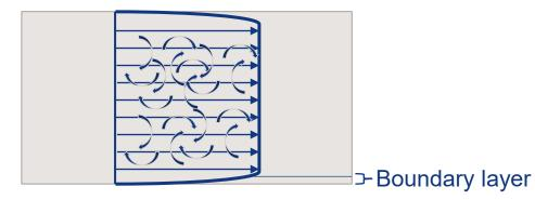
Re >4 000 – Turbulent flow Higher shear forces
