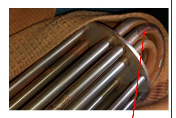
Bad bending makes SCC (Stress Corrosion Cracking)
