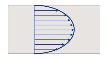
Re <4 000 – Laminar flow Low shear forces
