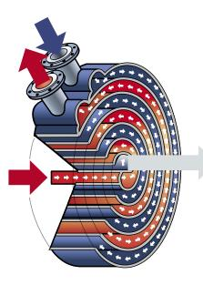
Above: Welded single-channel geometry eliminates the risk of intermixing of the two fluids.
