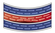
pressure drop increases pushing the fluid to find alternative flow paths. The result is that fouling and clogging of the tubes happens very quickly.
