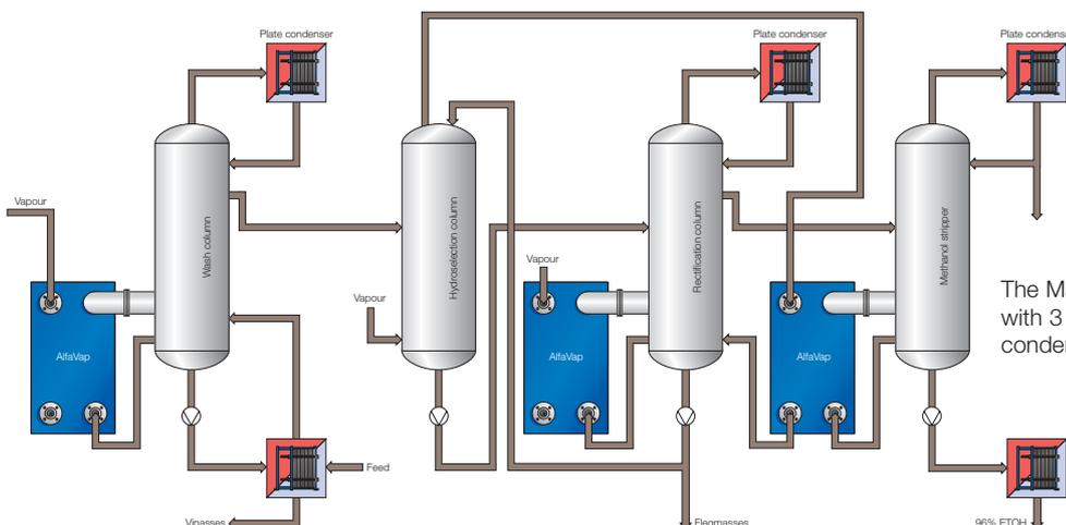
The Marconnelle distillation line is equipped with 3 AlfaVap reboilers in addition to plate condensers.
