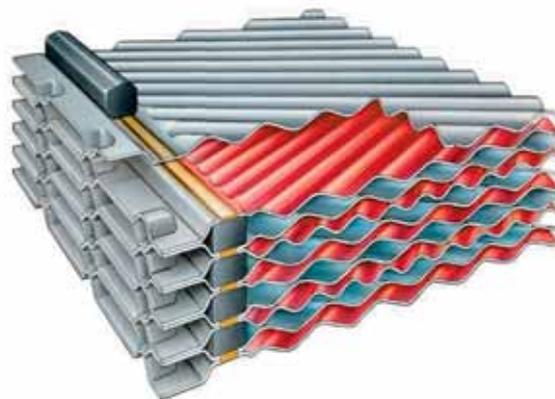
AlfaVap plates are welded in pairs to form cassettes separated by gaskets that are stable and durable even in high temperatures.
